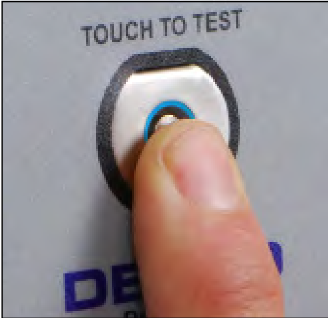
Figure 9. Bridging the test switch's contacts to initiate the test
